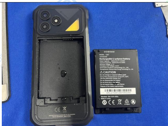
Fig.38: Disassembly Inspection after test
