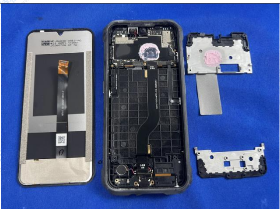
Fig.29: Disassembly Inspection after test
