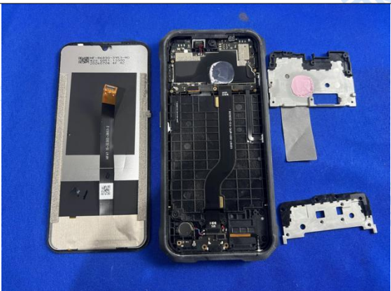
Fig.18: Disassembly Inspection after test
